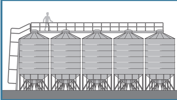
FIGURE 3 A platform with guard rails installed above silos
